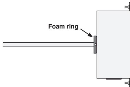
A 4" (102 mm) flange mounted on the electrical box has two holes to (not included) to fasten the sensor to the duct.
