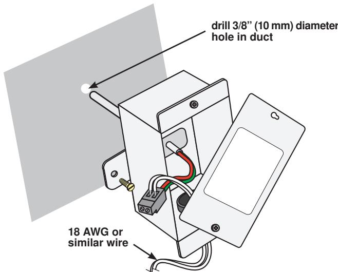
Ensure that the foam ring on the electrical box around the probe fits tight against the duct.
