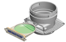
Air Intake Filter (installed)
