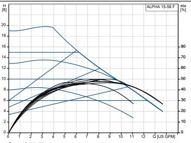
Pumped liquid = Water Liquid temperature during operation = 140  $^{\circ}$ F Density = 61.35 lb/ft³
