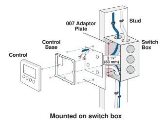
If a switch box was not used, mount the control directly to the wall.
