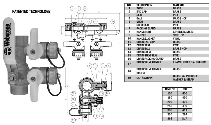
**Specifications**: Suitable for residential, commercial or industrial use with water or oil, this valve was specifically designed for filling and draining glycol/antifreeze from any point in a hydronic system. This approved Webstone valve is actuated by a blowout proof stem and features an adjustable packing gland. Threaded ends comply with ANSI B1.20.1.
