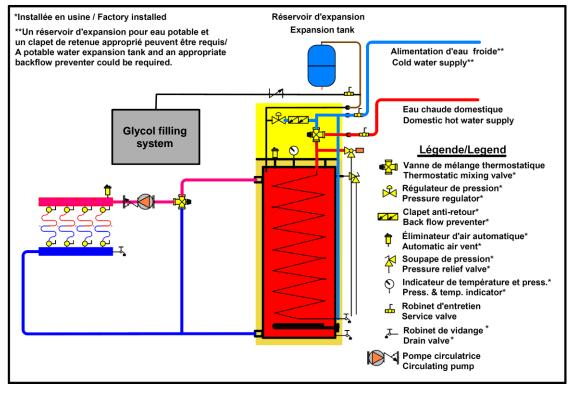
Figure 7: Installation drawing for radian floor with glycol filling system
