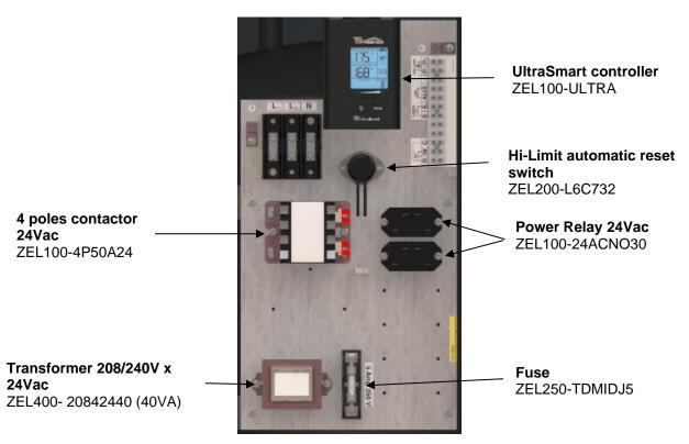
Figure 17: Electrical panel - Combomax Ultra 12 kW
