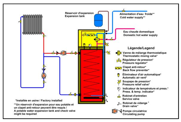
Figure 5: Installation drawing for radiators.
