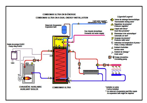
Figure 6: Installation drawing in dual-energy
