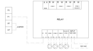
Figure 8: Multiple pump system with all zones wired and free ZC ZR terminals (total current less than or equal to 5A)
