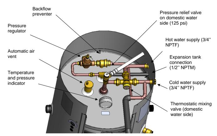
Figure 2: Components identification and location (Upper Compartment)
