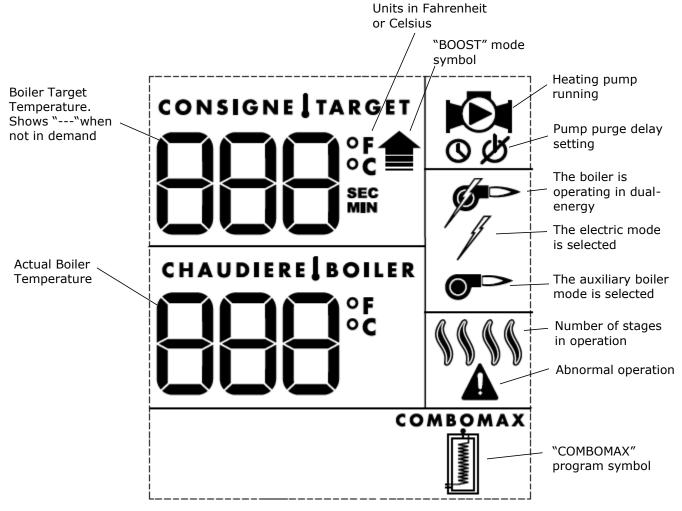
Figure 13: UltraSmart Controller Display
