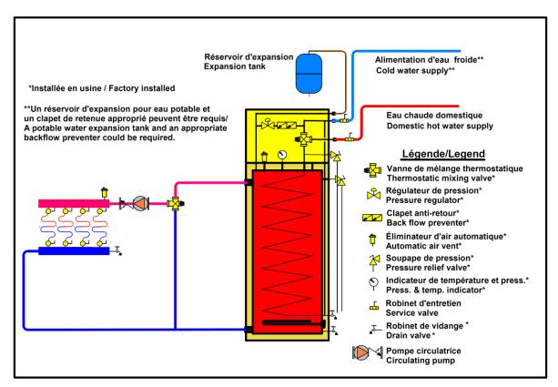
Figure 4: Installation drawing for radiant floor.
