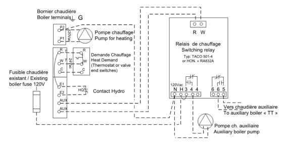
Figure 12: Wiring diagram in Dual-Energy
