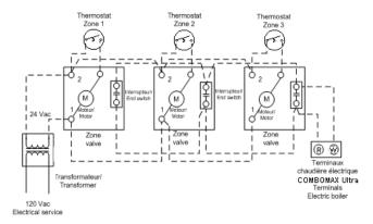
The 24 Vac power supply transformer used must be powerful enough to supply simultaneously all zone valves.
