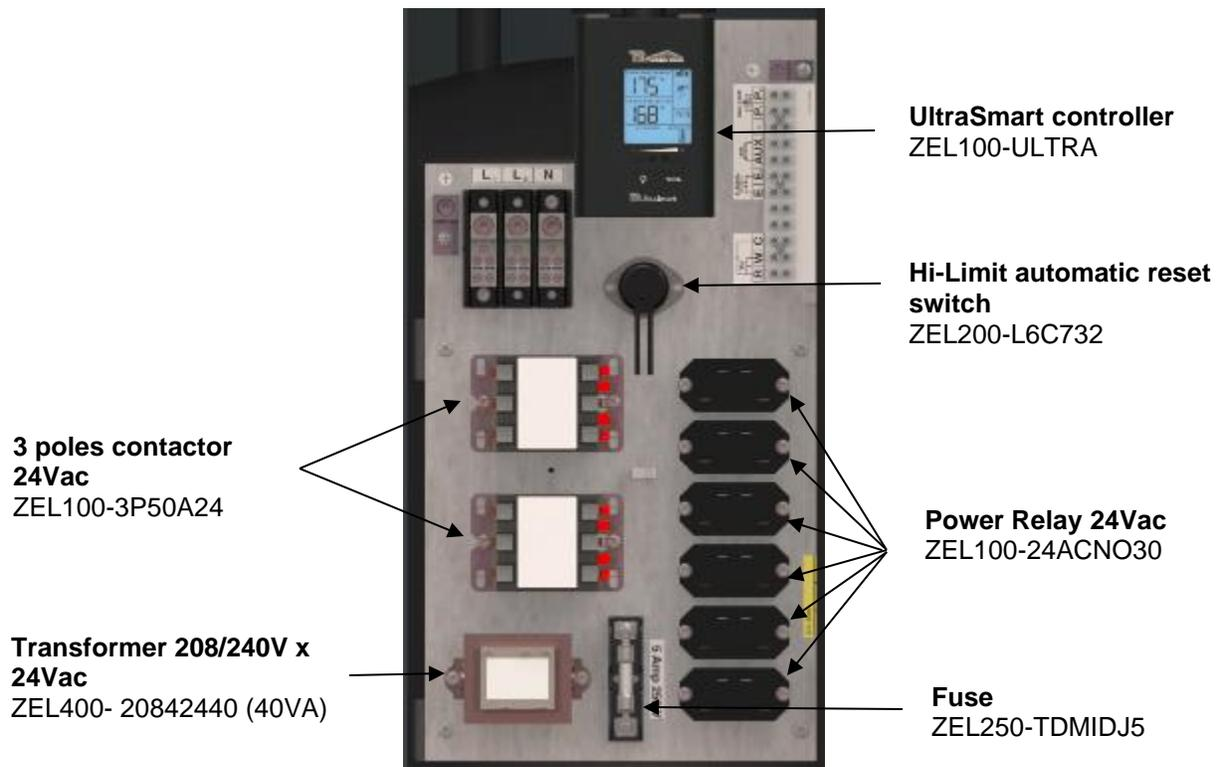
Figure 19: Electrical panel - Combomax Ultra 27 & 29 kW
