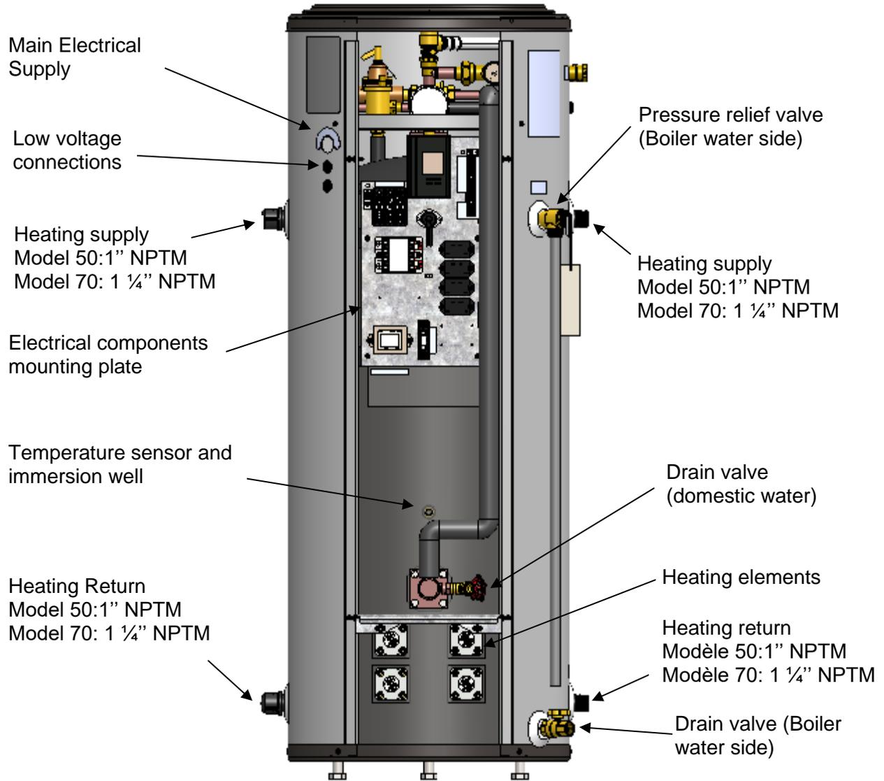
**Figure 3: Components identification and location (Front Compartment)**
