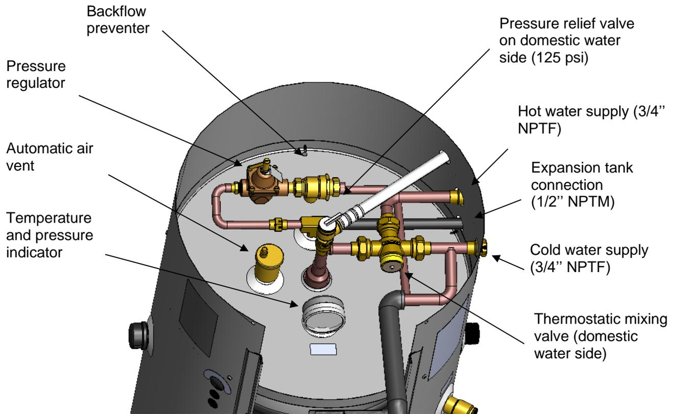
**Figure 2: Components identification and location (Upper Compartment)**
