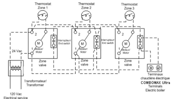
The 24 Vac power supply transformer used must be powerful enough to supply simultaneously all zone valves.
