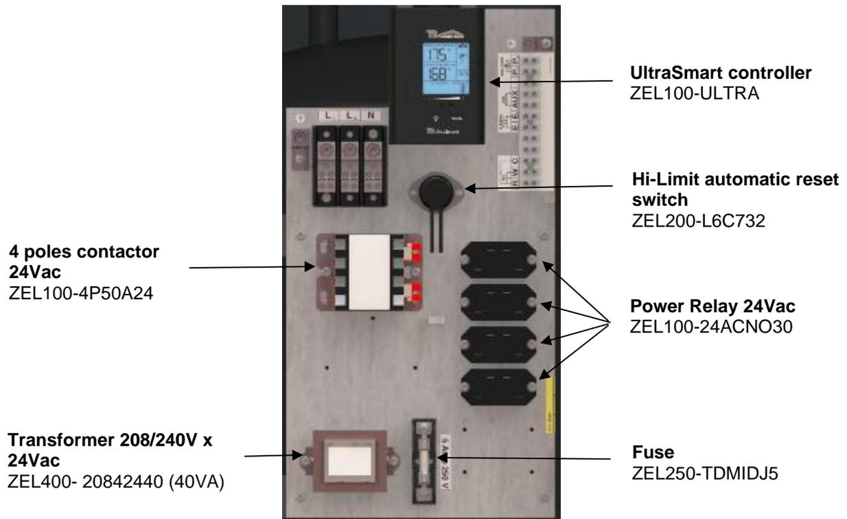
**Figure 18: Electrical panel - Combomax Ultra 15 to 24 kW**
