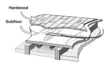
(45 mm) long should be cut to accommodate the sensor. The sensor should be located mid way between the heating elements to ensure a proper temperature reading.
