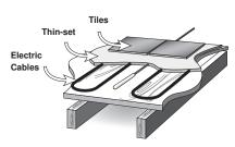
thin-pour should be avoided to ensure trouble free operation. The sensor should be located mid way between the heating elements to ensure a proper temperature reading.
