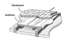
Splices under the floor covering should be avoided to ensure trouped and a groove 3/16" (5 mm) wide by 3/16" (5 mm) deep by 1-3/4" (45 mm) long should be cut to accommodate the sensor. The sensor should be located mid way between the heating elements to ensure a proper temperature reading.
