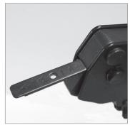
2. Use the Calibration Tool to gauge the jaw gap. The jaw gap should be between 1.2 mm and 1.4 mm.
