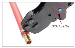
3. Place pinch clamp nub between tool jaws and ratchet the clamp (approximately seven times) until the LEDlight comes on. This will assure that the pinch clamp is fully engaged.
