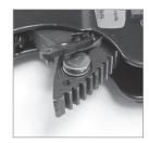
5. Place the new batteries with the positive side facing up.
