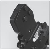
Ratchet the Pinch Tool to the closed position until the LED light comes on.
