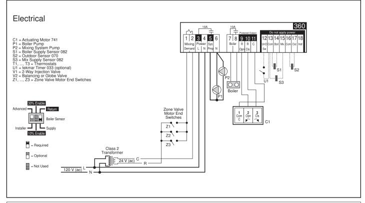
The Mixing Control 360 provides full outdoor reset to three (or more) mixed zones. The position of the injection valve is modulated to provide a mixed supply water temperature to the zones, and protect the boiler from flue gas condensation. The boiler operates at the required temperature in order to satisfy the load.
