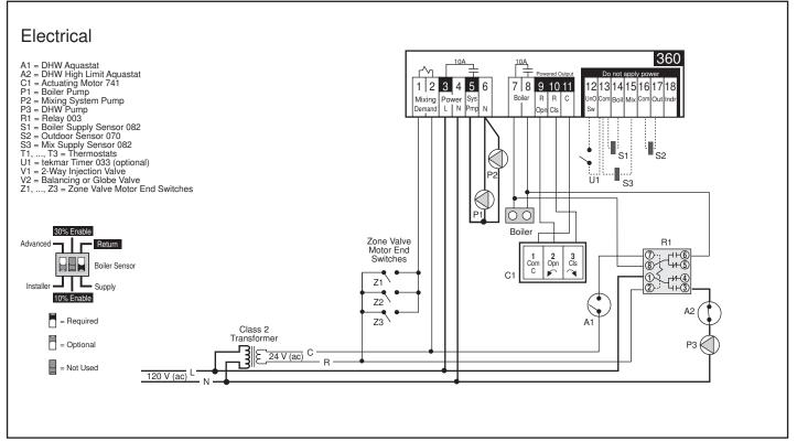
The Mixing Control 360 provides full outdoor reset to three (or more) mixed zones. The position of the injection valve is modulated to provide a mixed supply water temperature to the zones, and protect the boiler from flue gas condensation. The boiler operates at the required temperature in order to satisfy the loads. The supply of heat to an indirect Domestic Hot Water (DHW) tank is controlled through an external relay.
