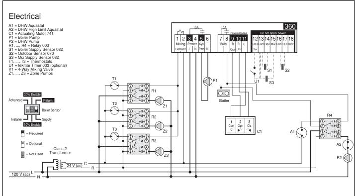
The Mixing Control 360 provides full outdoor reset to three (or more) mixed zones. The position of the mixing valve is modulated to provide a mixed supply water temperature to the zones, and protect the boiler from flue gas condensation. The boiler operates at the required temperature in order to satisfy the loads. The supply of heat to an indirect Domestic Hot Water (DHW) tank is controlled through an external relay.
