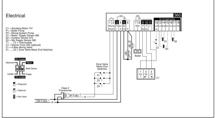
The Mixing Control 360 provides full outdoor reset to three (or more) mixed zones. The position of the mixing valve is modulated to provide a mixed supply water temperature to the zones, and protect the boiler from flue gas condensation. The boiler operates at the required temperature in order to satisfy the load.
