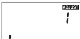
Press and release the *Item* button to advance to the *Terminal Unit* adjustment. Use the ▲ or ▼ button to select the desired terminal unit. The terminal unit number corresponds to the type of terminal that is being used. The table below lists the terminal units and their default values.
