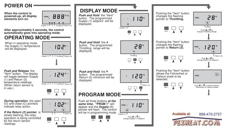
The control automatically goes back to operating mode when the buttons are left alone for 20 seconds -
