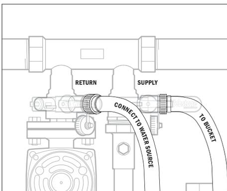
11. Connect system return purging valve hose to a water source.
