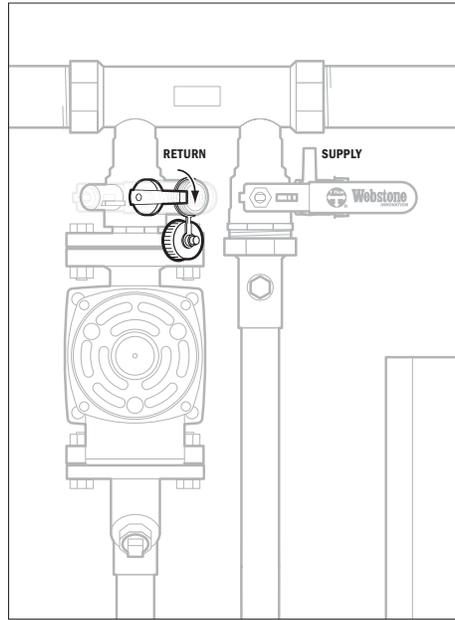
2. Release internal pressure by removing the system return purging valve cap and turning the drain handle on the system return purging valve into the open position (parallel with the flange). Pressure release should emit a small amount of fluid.
