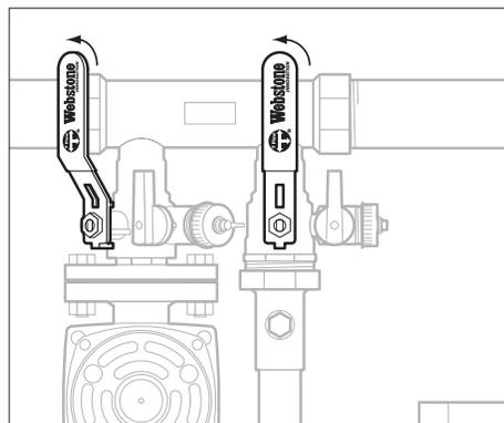
10. Return the lever handled ball valves to their normal operating position (handles perpendicular to the flange).
