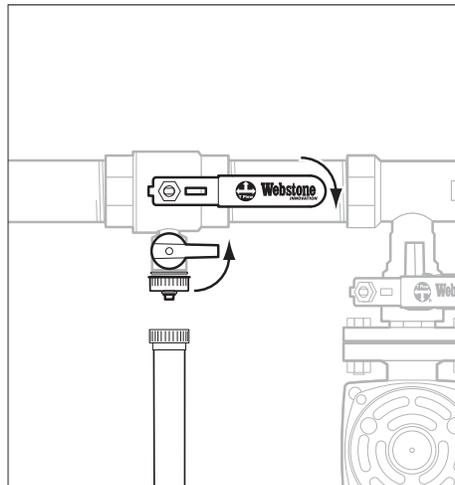
**8.** Close the purging valve on the drain in the secondary loop.
