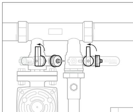
14. Close the two purging valves, remove the hoses, and replace the caps.
