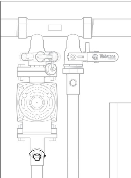
5. Reinstall the plug, ensuring that it is seated properly in the strainer cap.
