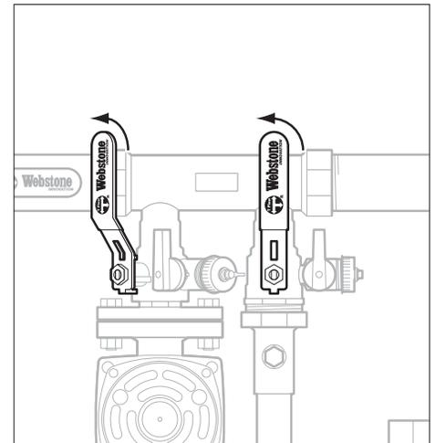
**11.** Return the lever handled ball valves on the Hydro-Core manifold to their normal operating position (handles perpendicular to the flange). Repeat for each circuit.
