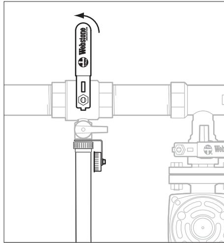
**2.** Close the main valve and remove the cap from the drain valve in the secondary loop.
