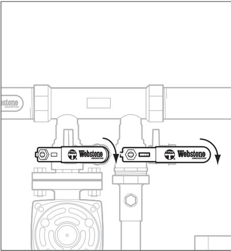
**1.** Turn the lever handles on both Hydro-Core ball valves so that they are parallel to the flange and the main valves are in the closed position. This will prevent any debris from entering the near boiler loop during flushing. If multiple circuits are present, repeat for each circuit.
