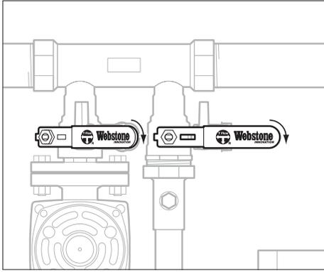
1. Turn the lever handles on both Hydro-Core ball valves so that they are parallel to the flange. The T-Flow handle logo indicates the flow pattern inside the valve. The logo should indicate that flow can go through the purging valve and both the supply and return piped assemblies.
