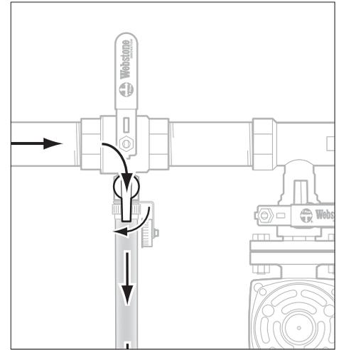
**5.** With the main water supply on and flowing into the system, open the purging valve on the drain in the secondary loop.
