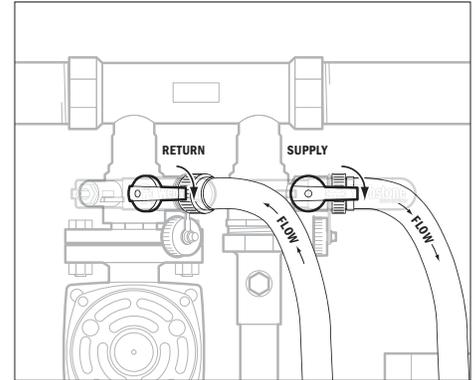
5. Turn the drain handles on both the system return & system supply purging valves into the open position (drain handles parallel with the flange).
