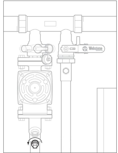
3. Remove the strainer plug by turning it counterclockwise.
