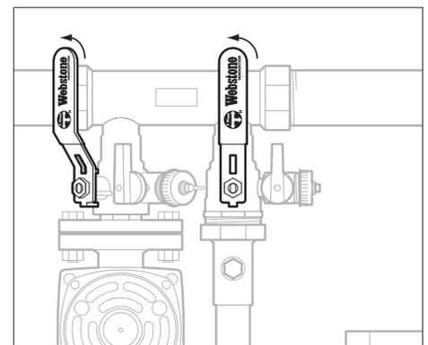
16. Return the lever handled ball valves to their normal operating position (handles perpendicular to the flange).
