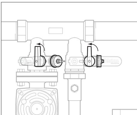
8. Once the air has been purged out and the drainage runs clear, turn off the circulator, close the two purging valves, remove the hoses, and replace the drain caps.
