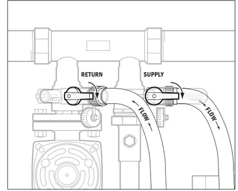
7. Turn the drain handles on both the system return & system supply purging valves into the open position (drain handles parallel with the flange).
