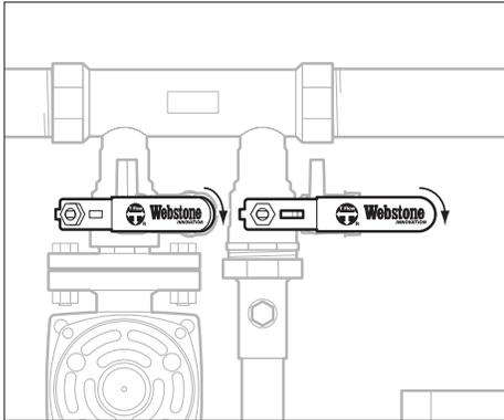
1. Turn the Lever Handles on both Hydro-Core ball valves so that they are parallel to the flange. The T-Flow handle logo indicates the flow pattern inside the valve. The logo should indicate that flow can go through the purging valve and both the supply and return piped assemblies.
