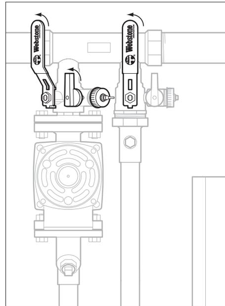
6. Close the purging valve (drain handle perpendicular to the flange).
