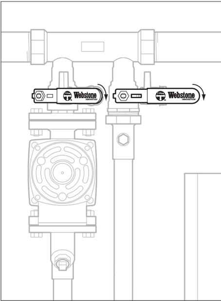
1. Turn the lever handles on both Hydro-Core ball valves so that they are parallel to the flange. The T-Flow handle logo indicates the flow pattern inside the valve. The logo should indicate that flow can go through the purging valve and both the supply and return piped assemblies.
