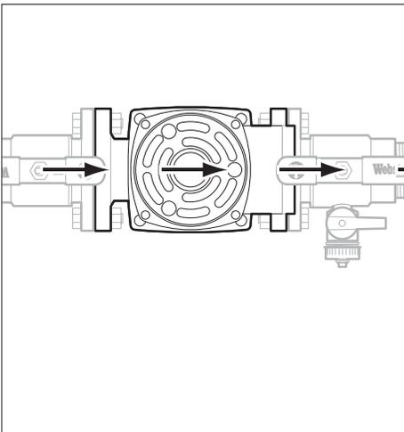
**6.** Turn on the circulator pump in the secondary system to purge the entire loop with fresh water.
