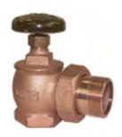
The T-431 Steam Angle Radiator Valve features a sturdy body made from cast bronze. The large screwed bonnet supports the rising stem and EPDM composition disc.
