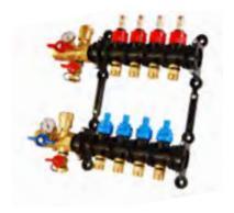
M-8100P EP Pro Manifold - Includes an integrated adapter valve with garden hose threads, fill & purge valve, automatic air vent, thermometer, isolation valve, and sensor port all in one unit.
