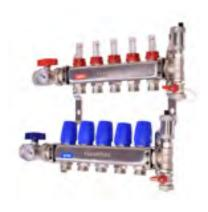
M-8330P Stainless Steel Manifold Pro – Features an automatic air vent, fill & purge adapter, and supply & return isolation valves with thermometers. 1" Supply and return headers.
