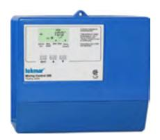
The Floating Actino Mixing Controller is designed to operate a mixing valve using Outdoor Temperature Reset. It can be used in applications ranging from in-floor radiant to commercial baseboard systems for Boiler Return Protection with full reset. This control regulates a single heating water temperature through Mixing Outdoor Reset. It controls the mixing by opening or closing a floating action type mixing valve actuator (3 or 4 way valves), and also provides control of the mix system pump.
