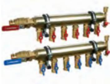
M-8220P High Capacity Manifold Press Kit – Base kit includes supply and return headers, 1-1/2" LegendPress® isolation valves for headers, 1" NPT circuit loop isolation valves for supply and return, mounting brackets, and fill & air purger.
