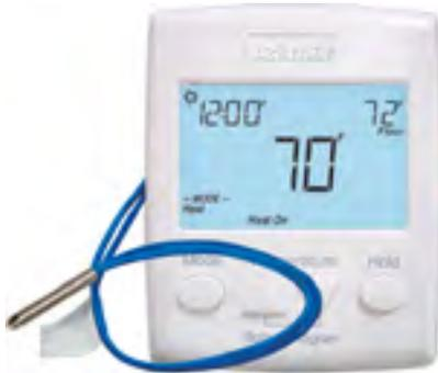
The Programmable Thermostat is designed for three different modes of operation: single stage heating, two stages of heating with a fan, or one stage of heating and one stage of cooling with a fan. Two auxiliary sensors may be added to measure the floor, outdoor or room temperature.
