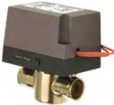
Zone Valves LZV-2 and LZV-3 series motorized valves are used to control flow in chilled or hot water systems and low pressure steam systems up to 15 psi. The valve is driven by a hysteresis synchronous motor with spring return.
