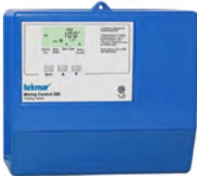
The Floating Actino Mixing Controller is designed to operate a mixing valve using Outdoor Temperature Reset. It can be used in applications ranging from in-floor radiant to commercial baseboard systems for Boiler Return Protection with full reset. This control regulates a single heating water temperature through Mixing Outdoor Reset. It controls the mixing by opening or closing a floating action type mixing valve actuator (3 or 4 way valves), and also provides control of the mix system pump.
