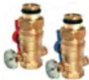
Substitute one or more multiple pairs of loop isolation valves with thermometer, in place of the standard loop isolation valves included with the manifold kits. The supply and return thermometer can provide means to determine delta T and help balance flow rates. Call customer service to make application adjustments (866) 752-2055.
