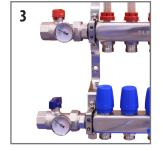
**Note:** These components seal together and to the manifold with an EPDM gasket (o-ring). One guarter (1/4) turn beyond "hand-tight" is normally sufficient to seal properly. If turning beyond 1/4 turn is required to align gauges and handles then do so, up to one (1) full turn beyond "hand-tight". Caution: Do Not use thread sealant tape or paste on these threads.
