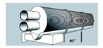
For this purpose, the pipe must be supported every 40" along its entire length because of the flexibility. To avoid bending, the pipe must be tied with straps to a supporting structure every 40".
