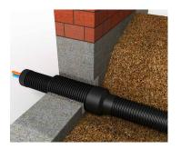
The annular space between the Terre-Pex pipe and the wall opening must be filled carefully.
