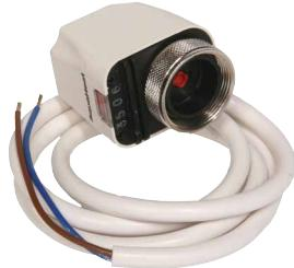
ProZone Actuators match the ProMix line of manifolds 2013xx/2015xx. 4 wire models include an end switch to operate a pump or other function only when actuator is fully opened. Operating temperature 32° F - 122°F, Power supply 24 VAC, Action is Open/Close, NC normally closed.
