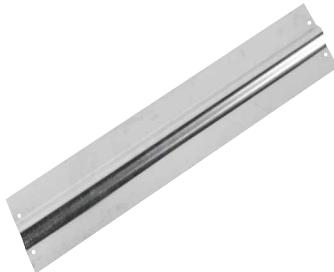
Heat transfer plates are used for Dry Below installations of 3/8", 1/2" or 5/8" pex. Plates provide a direct transfer and heat distribution from Pex piping to the underside of a wooden subfloor. HeatTrak simplifies the installation by allowing the pipe to be snapped in place.
