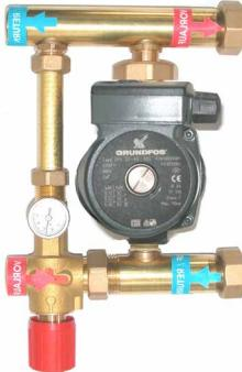
This ProMix manifold extension controls the 2013 series manifold supply water temperature by mixing supply and return water and limits the supply temperature flow through the manifold for e.d. wooden flooring. The integrated pressure by-pass relief allows to operate the manifold directly off a high-temperature primary heating circuit or boiler with a maximum heating capacity of 51,000 BTU/h.
