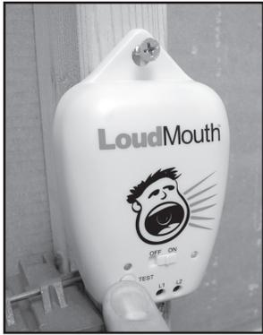
**The LoudMouth™ monitor shown at left will constantly monitor the heating wire during the entire installation process. If the wire is cut or damaged during installation, this device sounds an alarm. The LoudMouth will prevent burying a damaged wire below hardened concrete.**
