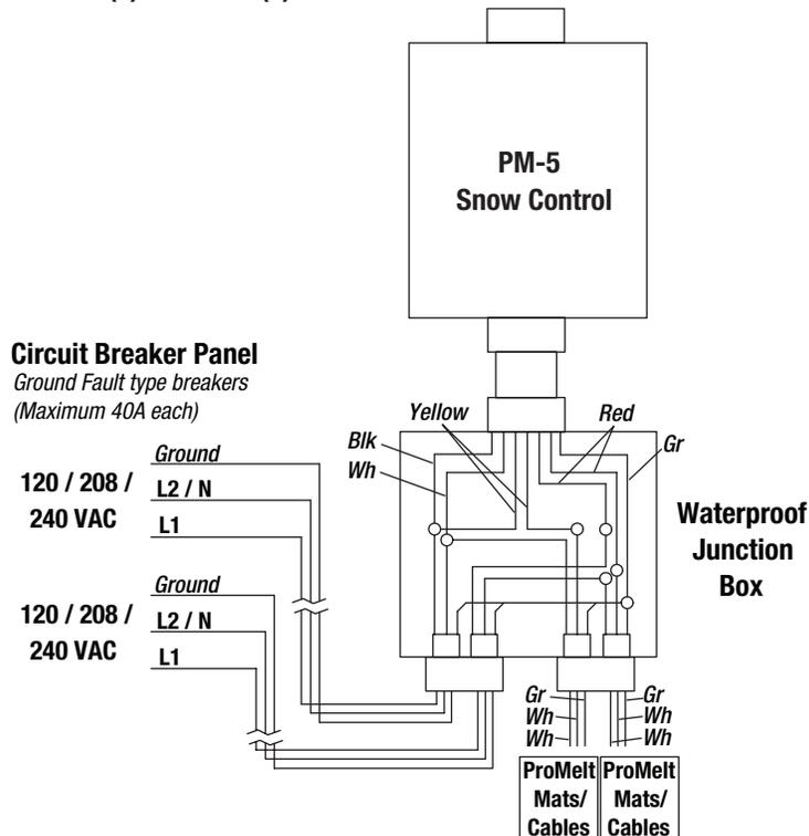
**ProMelt Snow Melting Control Kit PM-L3 with ProMelt Mat(s) or Cable(s)**
