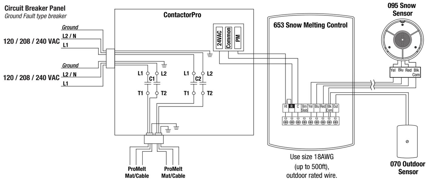
ProMelt Snow Melting Control Kit PM-L1 with ProMelt Mat(s) or Cable(s)
