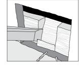
For retrofit installations. cut out drywall and chisel out the bottom plate to route wires to control.
