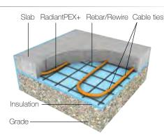
Install RadiantPEX+ in slab systems for radiant floor heating applications.
