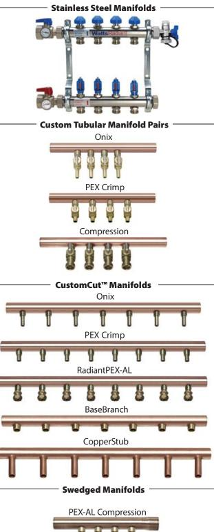
Stainless Steel manifolds are made of heavy-walled stainless steel. Matching fittings and accessories are made of solid brass and are heavily plated with nickel to match the appearance of the manifold trunk. Standard features included flow balancing valves, circuit isolation valves, and flow meters. Manifolds are sold in pre-mounted pairs in 1" and 1 1/2" sizes.
