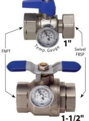
**Transitional Trunk Isolation Ball Valves with Temperature Gauge** — provides manifold isolation and transition to NPT threads.
