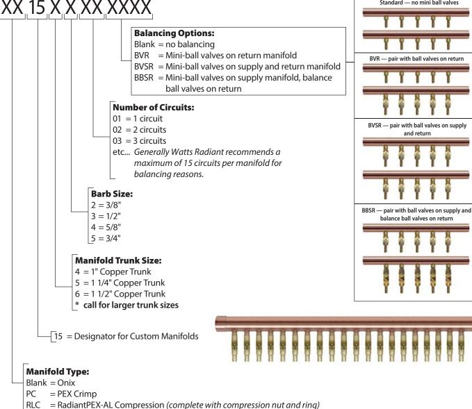
Ordering examples: •PC156410BVR= 10 branch, 1-1/2" trunk, 5/8" PEX Crimp manifold with mini ball valves on return •154207BBSR= 7 branch, 1" trunk, 3/8" Onix manifold with mini ball valves on supply and balance valves on return
