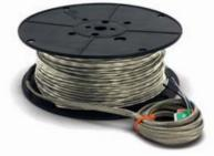
• Evaluate how many square feet of floor to be heated. Do not put under cabinets or appliances. Generally, about 85–90% of the open areas should be heated. Leave the wire at least 6" away from the toilet wax ring and 4"–6" away from your walls. To keep toes warm, install right up to the toe-kick in front of kitchen or bath cabinets, and in front of a toilet, shower, or tub.
