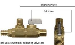
useful for exact flow balancing. Balancing is accomplished by rotating the threaded spindle below the brass safety cap. Each turn represents approximately 10% of full flow.
