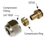
**SST20 PEX Compression Fittings** — for connecting PEX to Stainless Steel manifolds, and Custom Tubular T20 compression manifolds, or 3/4" male BSP x male sweat fittings.
