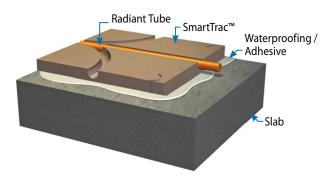
Concrete slabs which are attached to radiant heating systems should typically have insulation between the soil and the concrete along the edge (perimeter) and beneath. Recommended R-values vary with climate. Heating non-insulated slabs may increase heat loss and energy use.
