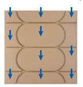
When using staples instead of screws it is very important that the board is glued and stapled with the same quantity of glue and staple points as shown in the pattern above. Cross stapling with a sheathing stapler is the fastest way to install SmartTrac<sup>™</sup>. 1-1/2" (38 mm) long, 16 gauge staples are recommended. Cross stapling means 2 staples are put closely together at opposing 45° angles. (45° angle to the surface)
