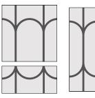
Various shapes can be cut from the Standard Panel to finish off areas of the room less than 24" (610 mm).
