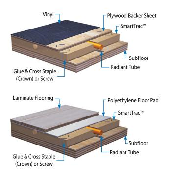
Prevent damage to laminate flooring by using controls that gradually adjust supply water temperatures with a reset curve. A floor temperature limiting sensor can be used to comply with flooring manufacturer's flooring temperature specifications.
