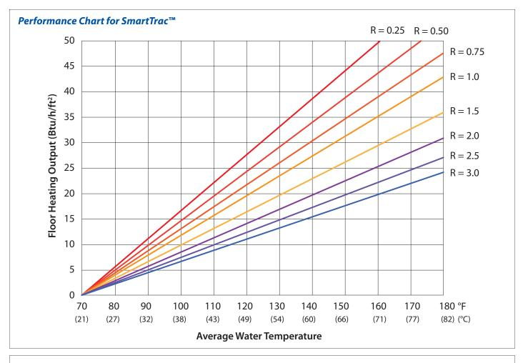
This chart shows average water temperature. In order to calculate required supply temperature, add half of expected delta-T to the average (i.e. add 10°F to the average if expected delta-T is 20°F).
