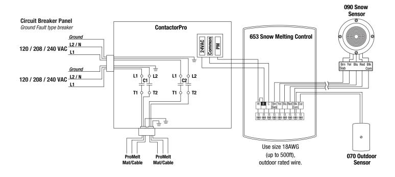
ProMelt Snow Melting Control Kit PM-L2 with ProMelt Mat(s) or Cable(s)
