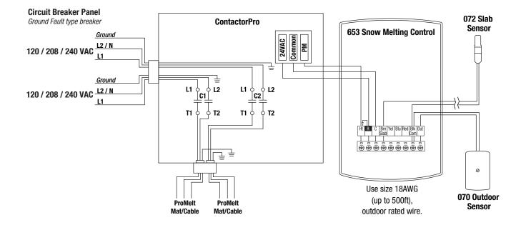
A separate, 120 VAC power supply is required for the ContactorPro internal transformer when using 277 VAC ProMelt Mats or Cables
