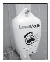
The LoudMouth<sup>™</sup> monitor shown at left will constantly monitor the heating wire during the entire installation process. If the wire is cut or damaged during installation, this device sounds an alarm. The LoudMouth will prevent burying a damaged wire below hardened concrete.
