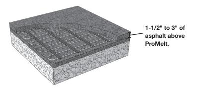
Compact the asphalt with a small power roller or compactor. Avoid using large power rollers which may compress aggregate into the cable. If possible, move the roller perpendicular with the cable direction to help avoid stress on the cable below. Be careful not to stop or start the roller over the mats as this could cause the asphalt to shift, potentially damaging the cables.
