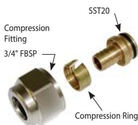
**SST20 PEX Compression Fittings** — for connecting PEX to Stainless Steel manifolds, and Custom Tubular T20 compression manifolds, or 3/4" male BSP x male sweat fittings.
