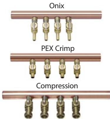
Watts Radiant **Custom Tubular manifolds** are manufactured to project specifications. All trunks are made of copper; all fittings and ball valves are brass. Every manifold is pressure tested before leaving the factory.
