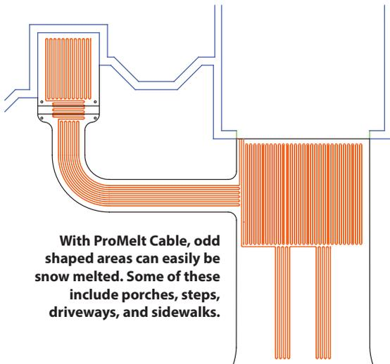
**With ProMelt Cable, odd shaped areas can easily be snow melted. Some of these include porches, steps, driveways, and sidewalks.**
