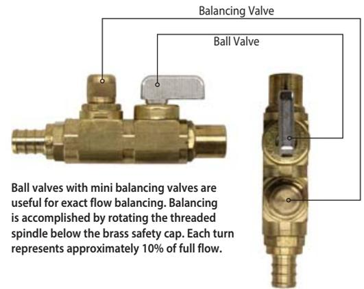
Ball valves with mini balancing valves are useful for exact flow balancing. Balancing is accomplished by rotating the threaded spindle below the brass safety cap. Each turn represents approximately 10% of full flow.
