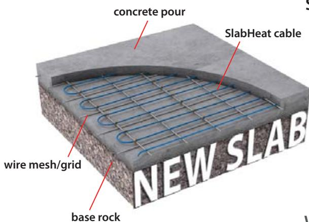
SlabHeat™ is engineered with the capability to produce enough BTUs to heat a slab, the space, and the surface people walk on. Regardless of size, shape, or thickness, SlabHeat is the way to provide heat to just about any environment.
