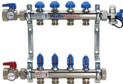
**Stainless Steel manifolds** are made of heavy-walled stainless steel. Matching fittings and accessories are made of solid brass and are heavily plated with nickel to match the appearance of the manifold trunk. Standard features included flow balancing valves, circuit isolation valves, and flow meters. Manifolds are sold in pre-mounted pairs in 1" and 1 1/2" sizes.
