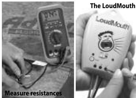
To retain the Limited Warranty, resistance readings and other data **MUST** be recorded in the Mat and Sensor Resistance Log below. Use the LoudMouth (right) to monitor the mat during the entire installation process.
