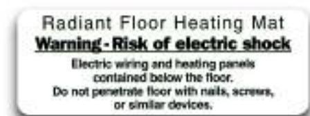
The Electric Radiant Heating Warning Label must be placed near, or on the face of the control.
