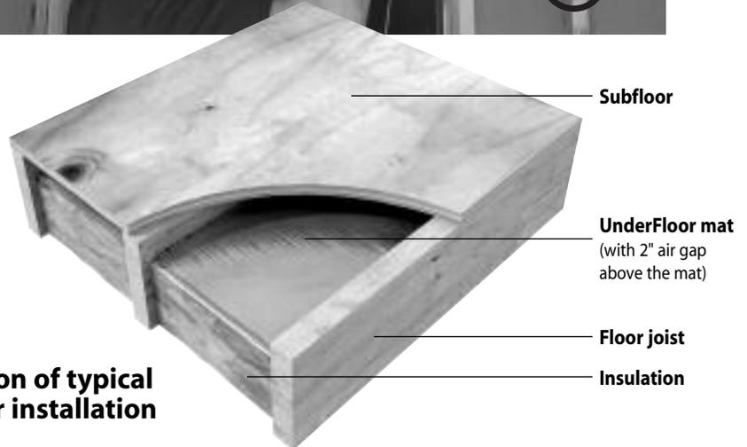
Cross section of typical UnderFloor installation
